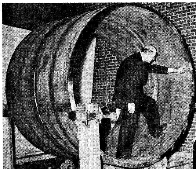
Fig. 11 Completed titanium cylinder 7 ft in diameter, 5 ft long and 6000 lb in weight.
